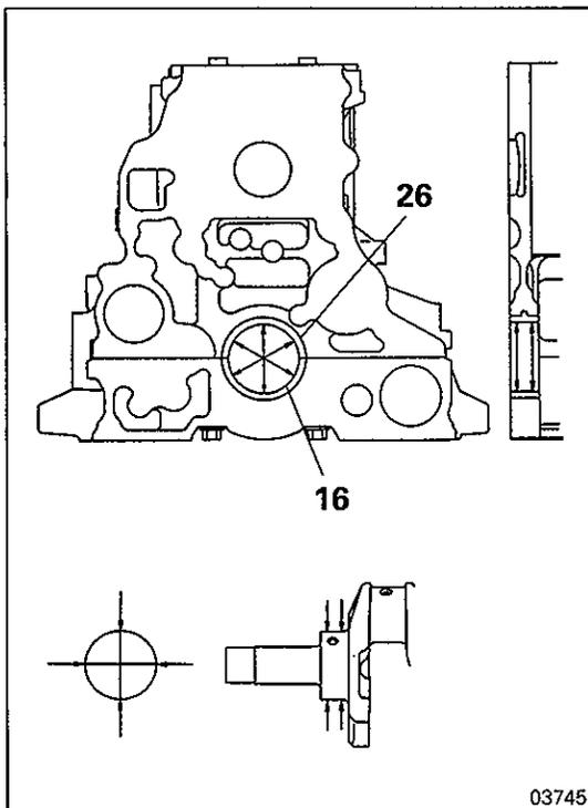
**Main Bearing-to-Crankshaft Clearance**
