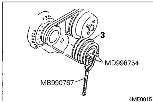
**REMOVAL SERVICE POINTS****◊A◊ CRANKSHAFT CENTER BOLT REMOVAL**
