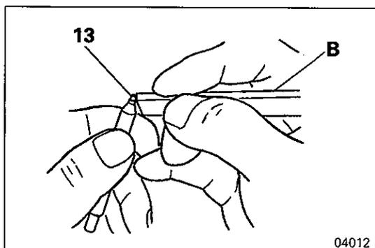
**CLEANING****NEEDLE VALVE / NOZZLE TIP**
