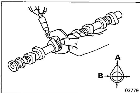
**Difference between Cam Height and Base Circle Diameter**
