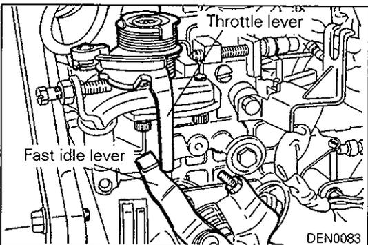
**FUEL INJECTION TIMING CHECK AND ADJUSTMENT**
