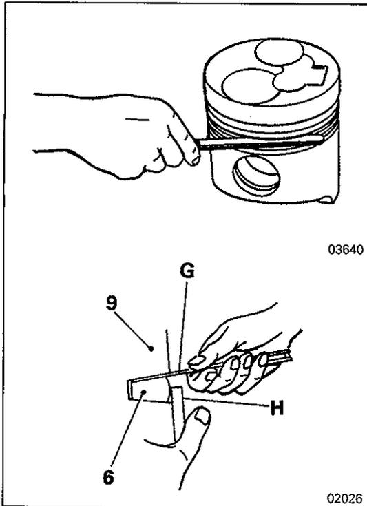
**PISTON RING TO PISTON RING GROOVE CLEARANCE**
