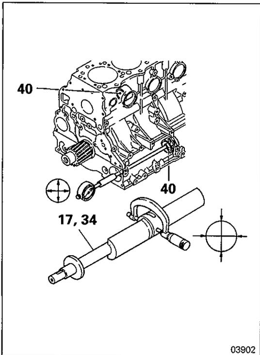
**BALANCE SHAFTS RH AND LH, AND BALANCE SHAFT BUSHES**
