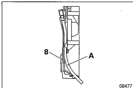
**◊B◊ TIMING GEAR CASE REMOVAL <L200>**
