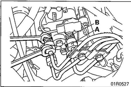
**◆C◆ FUEL INJECTION PIPE INSTALLATION**
