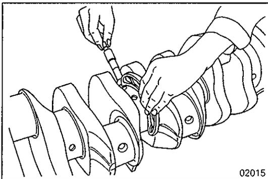
**INSPECTION****CRANKSHAFT****Out-of-Roundness and Conicity of Crankshaft Journal and Pin**
