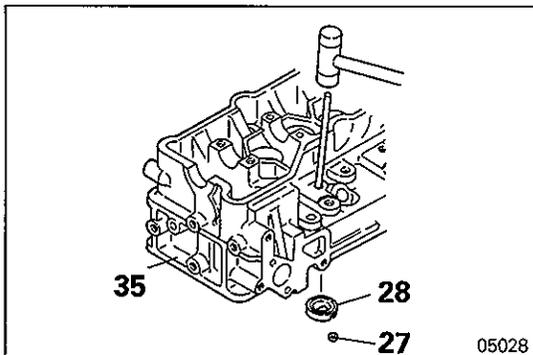
**◁D▷ TABLET/COMBUSTION JET REMOVAL**
