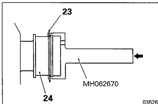
**INSTALLATION SERVICE POINTS****▶▶ REAR OIL SEAL SLINGER INSTALLATION**
