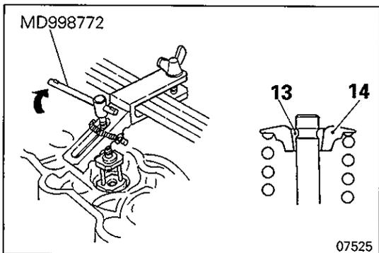
(3) Press down the upper retainer **14** and install the valve cotters **13**.
