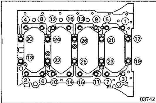
**REMOVAL SERVICE POINTS****◇A◇ BOLT / MAIN BEARING CAP BOLT REMOVAL**① – ⑯: Bolt **14**⑰ – ⑳: Main bearing cap bolt **15**
