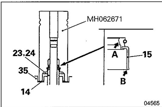
**▶G▶ VALVE STEM SEAL INSTALLATION**
