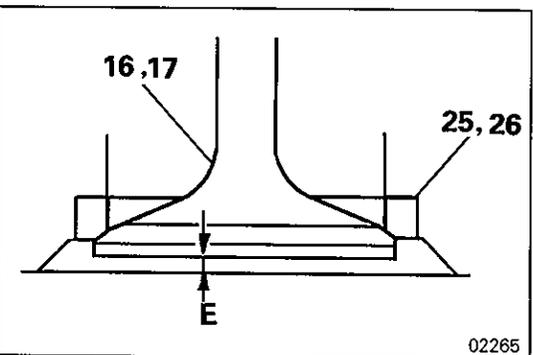
**Valve Sinkage from Cylinder Head Bottom**
